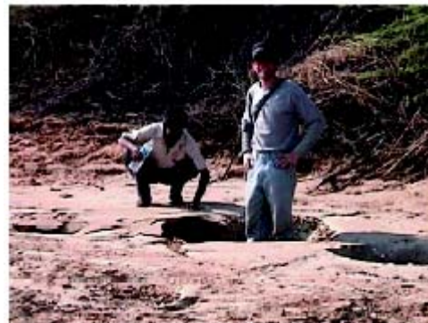
Figure 4.20: Sand-blow craters in a dry riverbed
