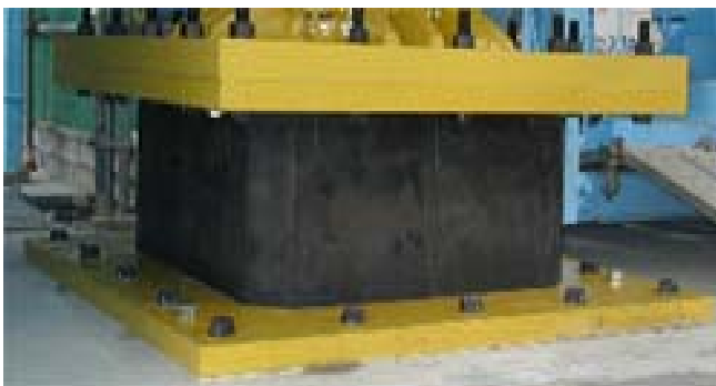
Figure 12.14: Rubber bearings with lead plugs
